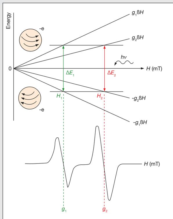
Figure A-1. Energy levels of two paramagnetic species with  $g$ -factors  $g_1$  and  $g_2$ . As the magnetic field  $H$  is increased the energy levels for the two species split at different rates, according to the Zeeman effect. Resonance occurs, and signals with derivative lineshapes are detected, when the energy separations ( $\Delta E_1$  and  $\Delta E_2$ ) are equal to the energy of the applied microwaves ( $h\nu$ ). From Ikeya (1993).
