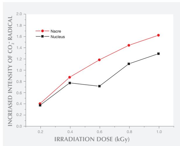
radiated spectrum (0 kGy, black line), the increased intensity of radicals was calculated by peak-to-peak height. The intensity of the  $\text{CO}_2^-$  radical is stronger in the nacre than in the nucleus when irradiated with a dose above 0.4 kGy (figure 7).
